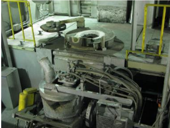
Fig.5 No.2 demonstration scale furnace (Capacity: 1ton-Fe/batch)
