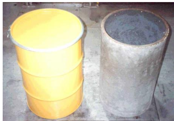
Fig.9 Metal Container made by centrifugal casting method
