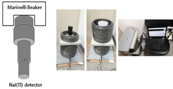
Fig. 5. Prototype of small liquid radioactivity (for gamma nuclide) measurement equipment using the 3inch NaI(Tl) detector and 1,000ml marinelli beaker
