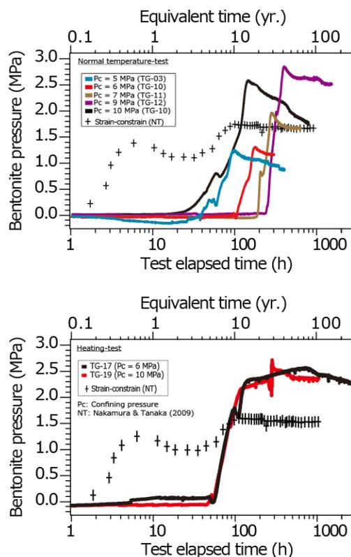
Fig. 5. Temporal change of bentonite pressure. (Upper) normal temperature-test, (lower) heating-test.
