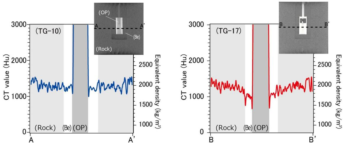
Fig. 6. Cross sectional image of the model by X-ray CT in the pre-test, (left) normal temperature-test, and (right) heating- test. Be: bentonite, OP: overpack.
