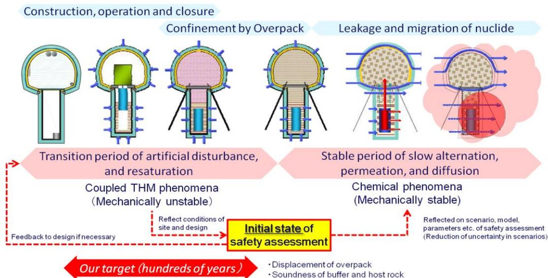
Fig. 1 Schematic of predictable transition in HLW geological disposal repository
