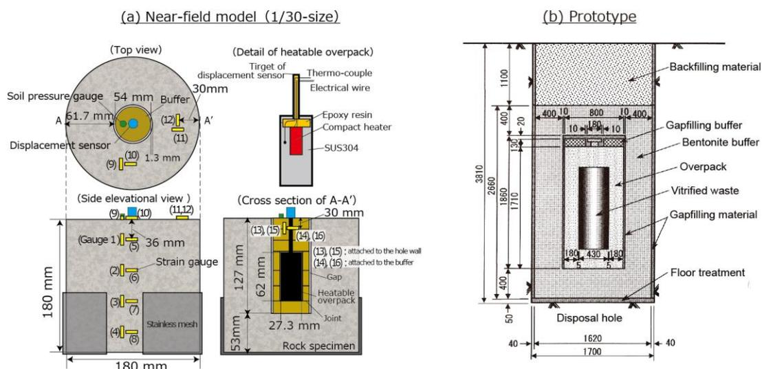
Fig. 3. (a) Near-field model of the centrifugal model test, and (b) the target HLW disposal repository.
