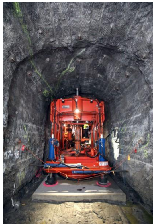
Fig. 2: Posiva's machine for boring disposal hole (source: Posiva).
