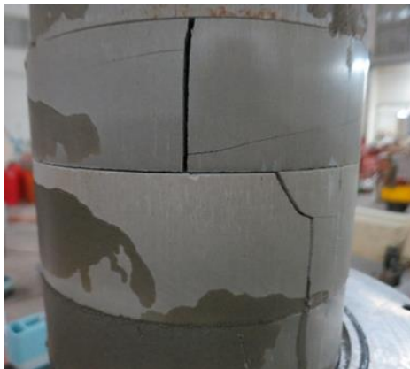
Figure 13: Cracking blocks and watermark (Model D-W24)
