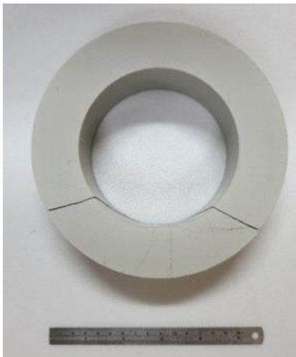
Figure 12: Cracks of buffer block (Model D-N)
