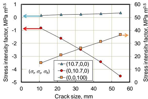
Fig. 7 Relationship between stress intensity factor and crack size in weld part for flat lid type
