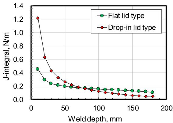
Fig. 5 Relationship between J-integral at tip of weld and weld depth
