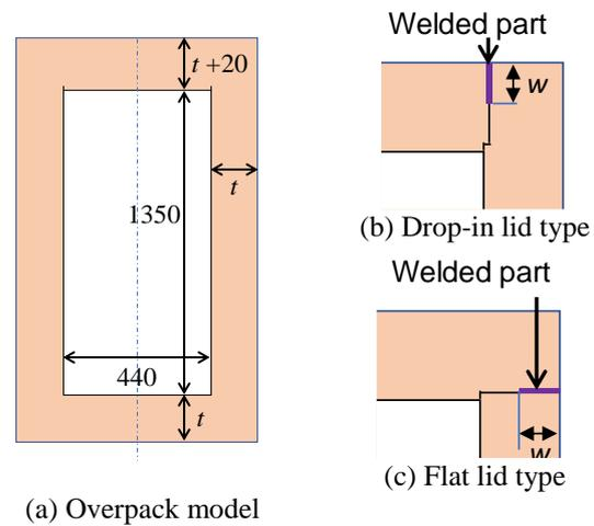
Fig. 2 Failure analysis model of overpack
