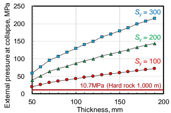
Fig. 3 Relationship between external pressure at collapse and thickness of overpack
