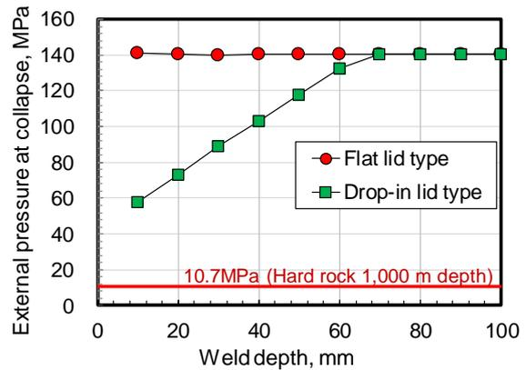
Fig. 6 Relationship between external pressure at collapse and weld depth (yield strength 300 MPa)
