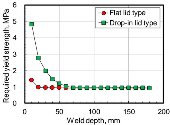
Fig. 4 Relationship between required yield strength and weld depth
