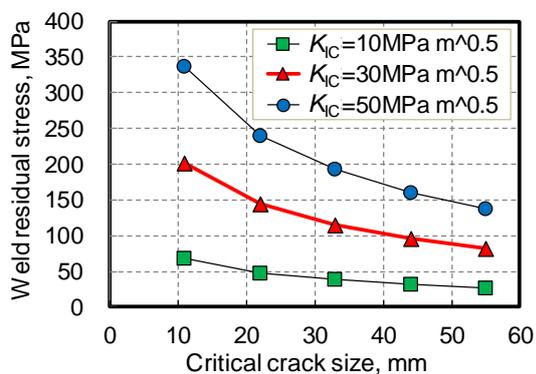
Fig. 8 Relationship between weld residual stress and critical crack size in weld part for flat lid type
