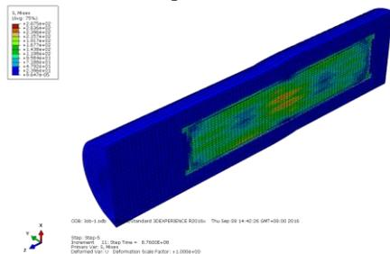
Fig. 6 Deformation and stress for assembly model imposed by 5cm shear displacement for 90° shear direction at middle section case
