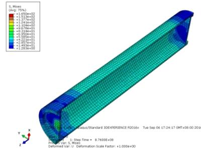
Fig. 8 Stress distribution of copper shell for 90° shear direction at quarter section case
