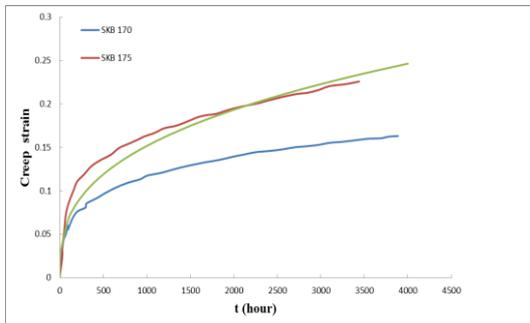
Fig. 3 Creep strain curve of copper matched by ABAQUS power-law creep model (green line)
