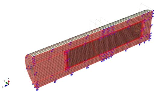
Fig. 1 Canister-buffer assembly model for 90° shear direction at middle section case
