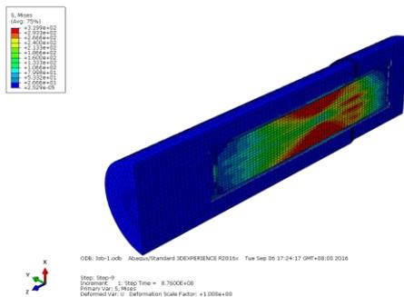
Fig. 4 Deformation and stress for assembly model imposed by 5cm shear displacement for 90° shear direction at quarter section case
