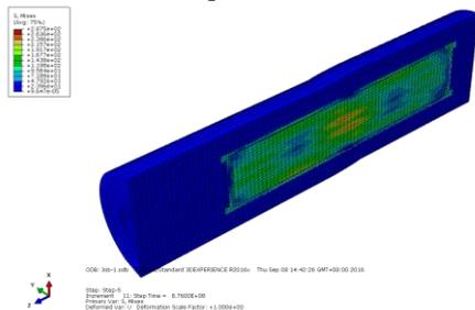
Fig. 6 Deformation and stress for assembly model imposed by 5cm shear displacement for 90° shear direction at middle section case
