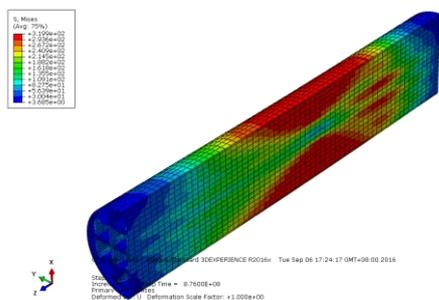
Fig. 7 Stress distribution of cast iron insert for 90° shear direction at quarter section case
