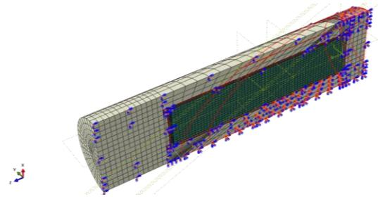
Fig. 2 Canister-buffer assembly model for 22.5° shear direction at middle section case
