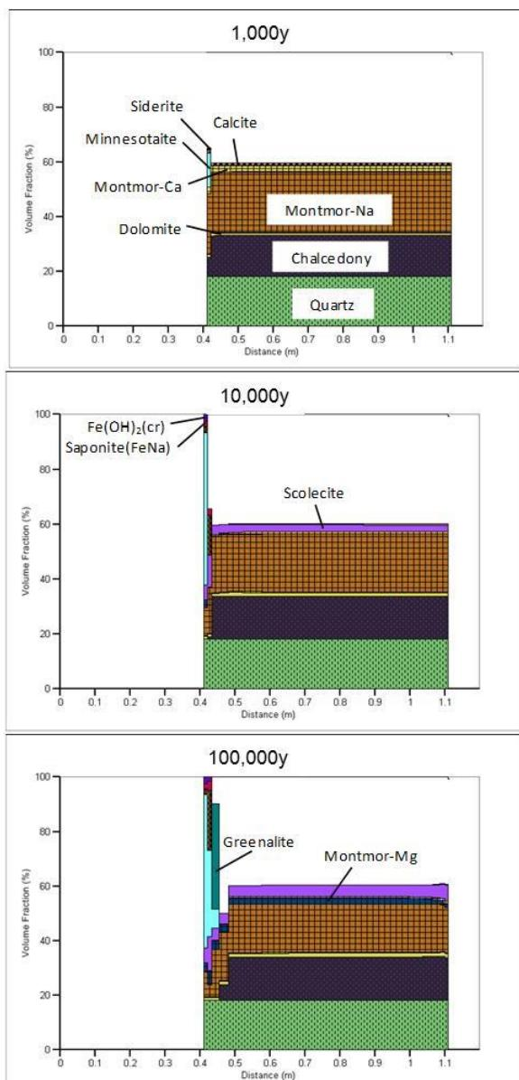
Figure 5 Bentonite alteration due to iron-bentonite interaction.
