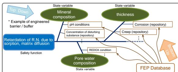
Figure 2 Structure of fishbone diagram
