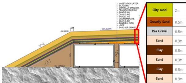
Figure 1. Configuration of multi-layer cover concept in the second stage LILW disposal facility
