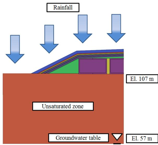
Figure 2. Concept model of ground water flow modeling for the second stage LILW disposal facility
