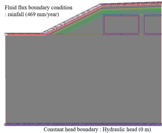
Figure 5. Applied boundary conditions for the calculation
