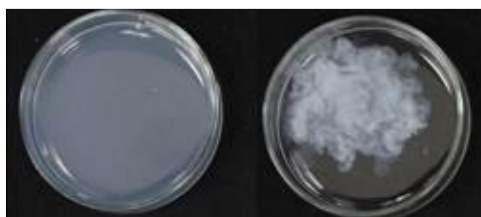
a) No turbidity, applicable b) Turbidity, not applicable Fig. 4: Turbidity check tests on sea water. It was performed during the grouting works at the Kurashiki LPG.
