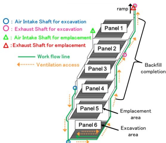
Fig. 2 DGR layout and ventilation access for the period of construction in sedimentary rocks.
