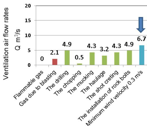
Fig. 6 Example of ventilation air flow rates at the time of excavation (crystalline rocks)
