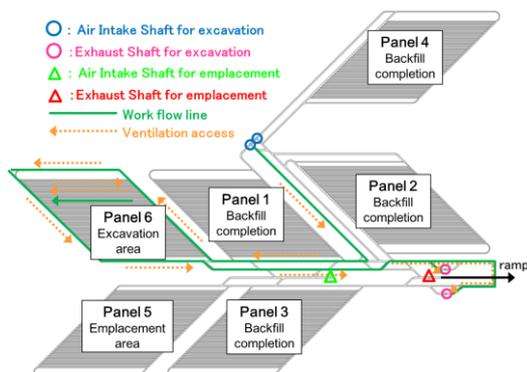
Fig. 1 DGR layout and ventilation access for the period of construction in crystalline rocks.
