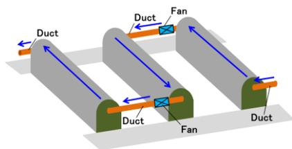
Fig.5 Ventilation access of a single stroke
