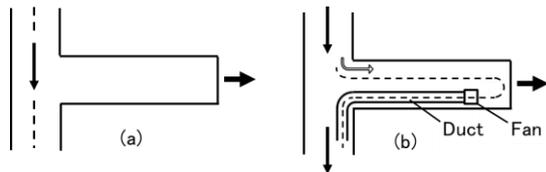
Fig. 4 Ventilation schematic illustration for dead-end tunnel [3]
