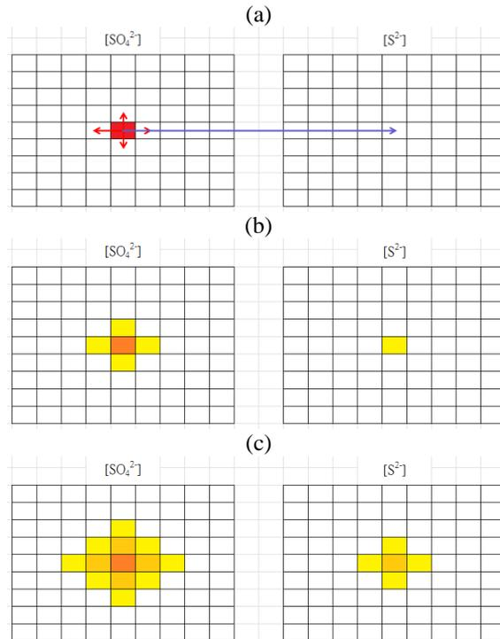
Figure 2-2 Illustrations of concept of the model. (a) Initial concentration contribution. Red arrows represent the transportation through diffusion; blue arrow represents SO<sub>4</sub><sup>2-</sup> reduction. (b) Concentration contribution after a time interval. (c) Concentration contribution after another time interval.
