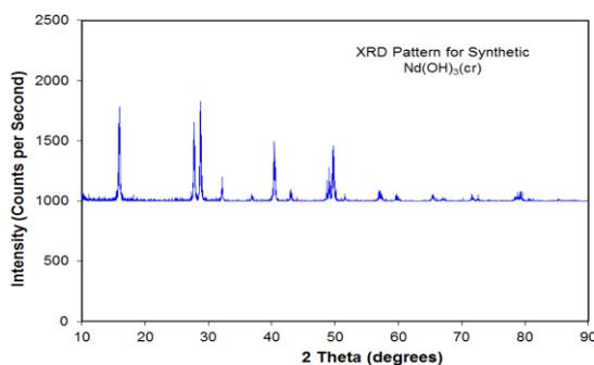
Fig. 2. XRD pattern of  $Nd(OH)_3(\text{micro cr})$  used in solubility experiments in this study.
