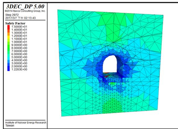
Figure 7. Safety factor for rock mass with 5 sets of DFN when normal period
