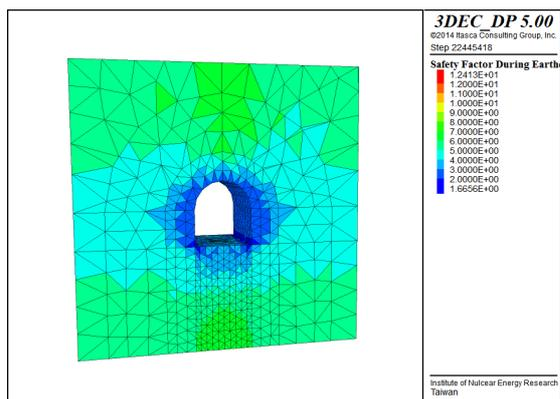
Figure 6. Safety factor for rock mass without fracture when earthquake period
