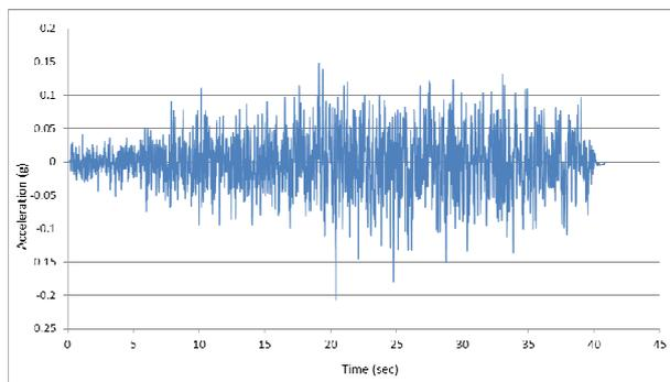
Figure 3. The input acceleration time history on the base of deposition tunnel model
