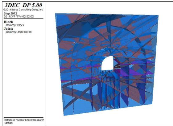
Figure 2. Tunnel model with 5 sets of DFN in rock mass
