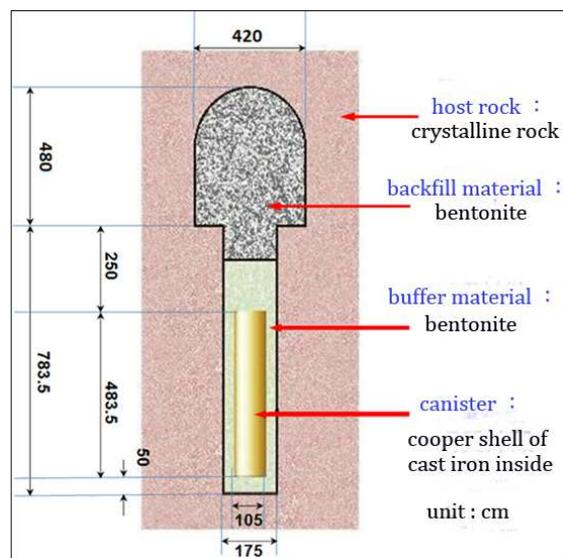
Figure 1. The cross section of disposal tunnel and disposal hole
