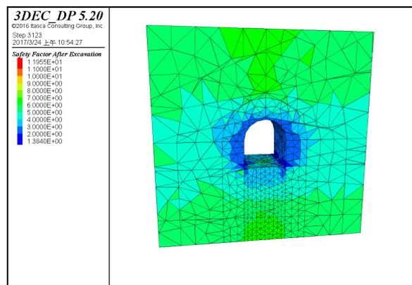
Figure 8. Safety factor for rock mass with 2 sets of DFN when normal period
