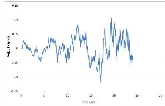
Figure 4. The input of velocity time history on the base of disposal tunnel model
