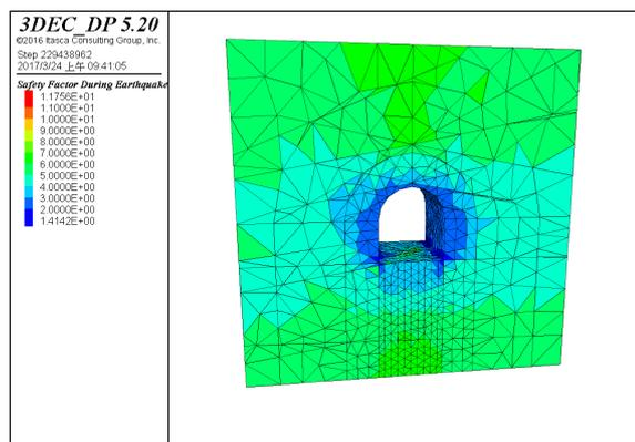
Figure 9. Safety factor for rock mass with 2 sets of DFN when earthquake period
