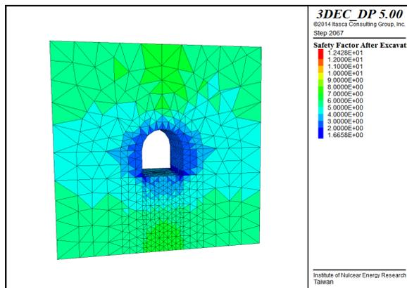
Figure 5. Safety factor for rock mass without fracture when normal period
