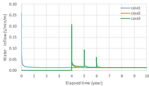
Figure 9 Changes in the amount of water inflow at the disposal tunnels
