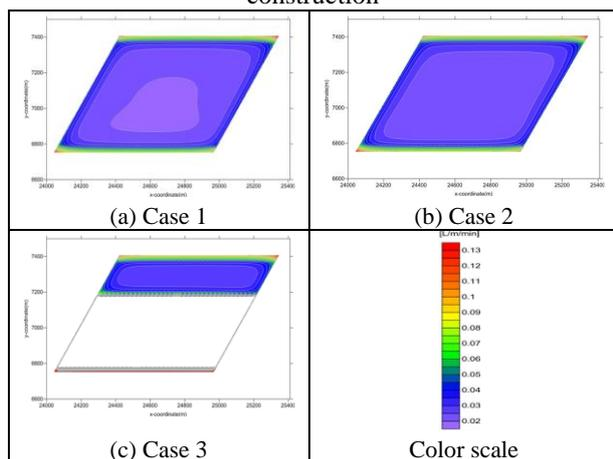
Figure 12 Comparison of disposal facilities water inflow volume due to differences in excavation process (5th year from excavation start)
