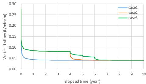
Figure 10 Changes in the amount of water inflow at the main tunnel
