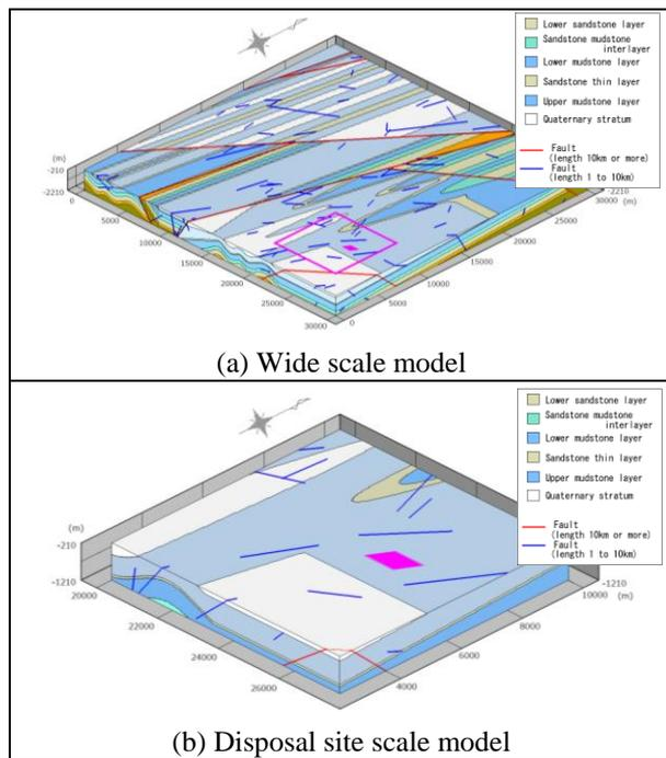
Figure 7 Hydraulic geological structure model of each scale (bird's eye view)
