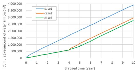
Figure 11 Changes in the total amount of water inflow at the disposal facility since the start of the construction
