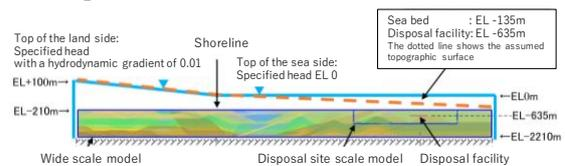
Figure 8 Boundary condition of the wide scale model
