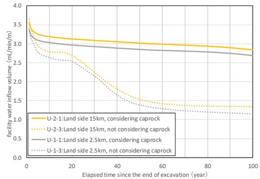
Figure 6 Change over time of the amount of water inflow at the disposal facility due to the caprock considered/not considered (in land)
