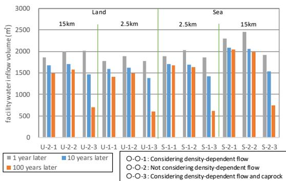
Figure 5 Comparison of the amount of water inflow at the disposal facility in each case
